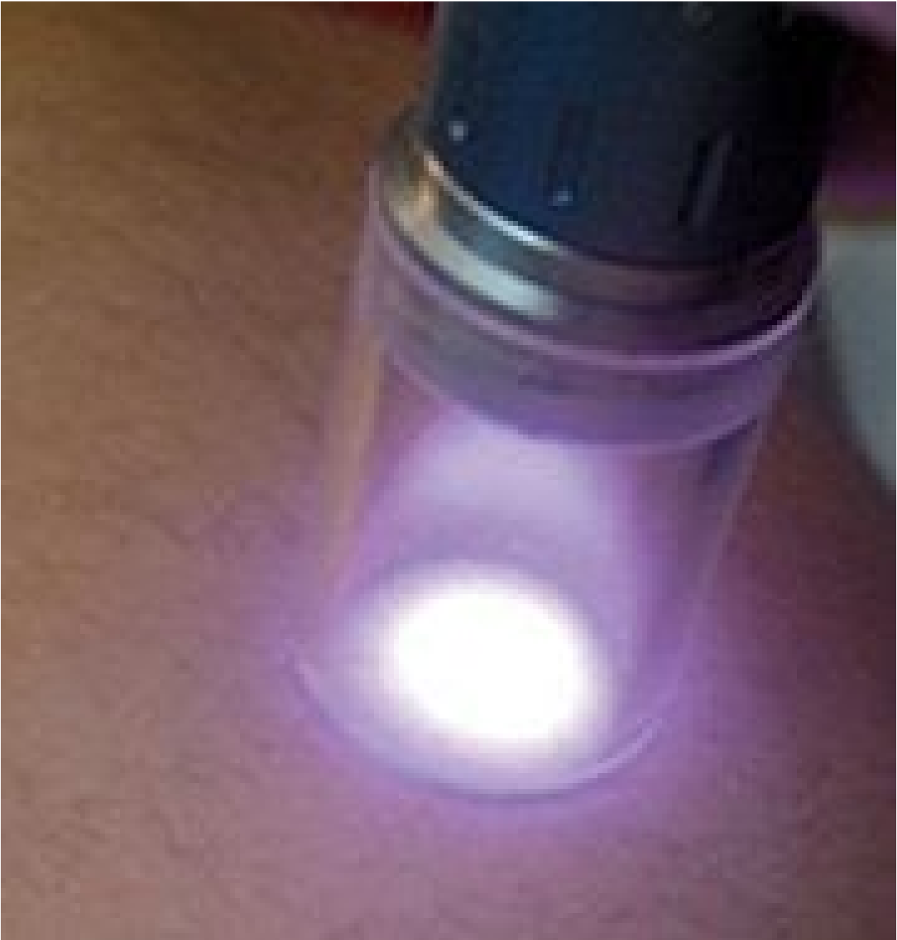
Figure 2: Class IV lasers use infrared wavelengths, which are invisible, but can be photographed with a digital camera.
