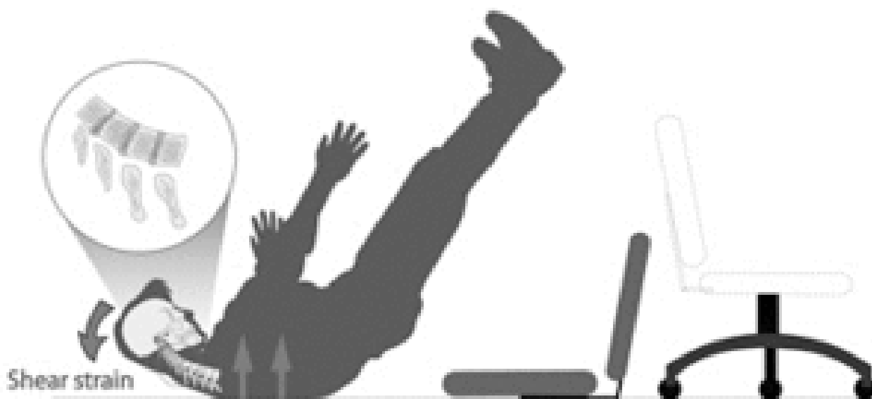
Figure 1. This illustration shows the broken chair and the first point of contact with the floor. It also illustrates that shear strain would have resulted as the thoracic spine was abruptly decelerated while the head's inertia carried it
