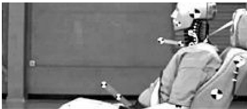
Figure 1. Late-model Ford Windstar head-restraint/seat-back test using BioRID dummy insimulated, 10-mph, rear-impact collision. This is the dummy position immediately prior to
