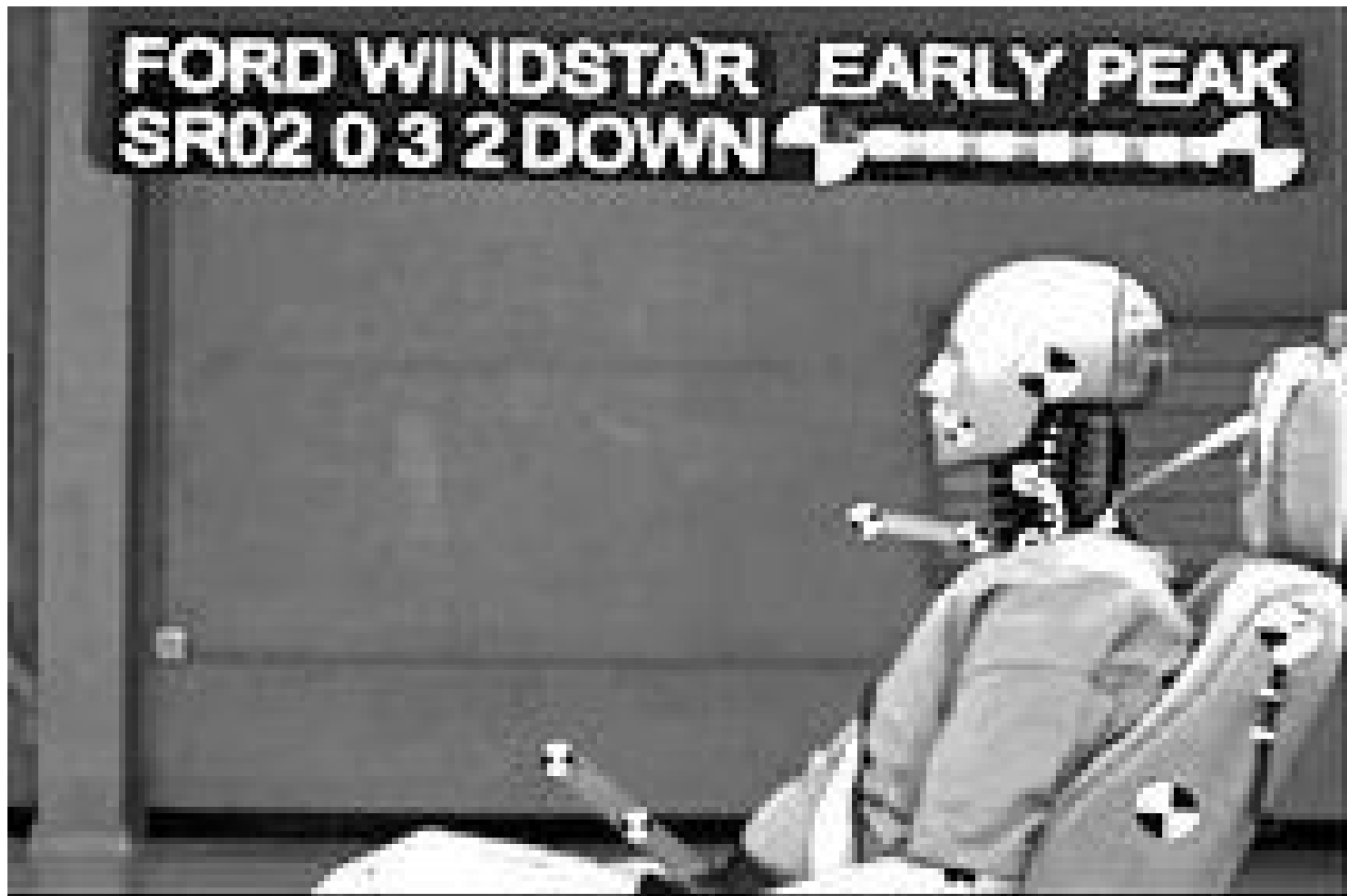
Figure 1. Late-model Ford Windstar head-restraint/seat-back test using BioRID dummy insimulated, 10-mph, rear-impact collision. This is the dummy position immediately prior to acceleration. The static geometry is marginal, but if the restraint were properly built, it still would be able to reduce significant shear and rearward bending movements to the neck.
